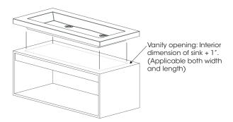
Figure #2 (Placing the lavatory)
